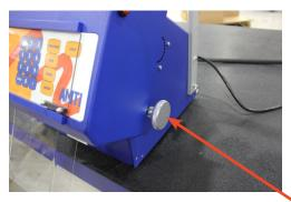
6. ADJUST BOTTOM GUIDE WHEEL APPROX. ¼" ON EACH SIDE OF MATERIAL
