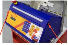
9. FEED MATERIAL INTO THE THROAT AND PRESS LH & RH ACTIVATION BUTTONS. MATERIAL WILL ADVANCE FOR ONE CUT CYCLE FOR LOAD SEQUENCE.
