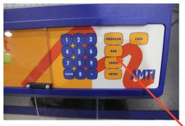
10. TO RUN: SLIDE KEYPAD SAFETY SHIELD TO LEFT. PRESS "RUN".
