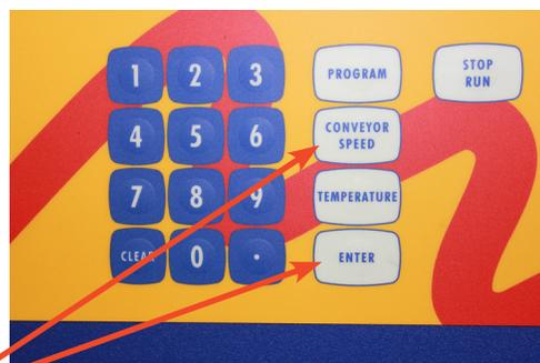
6. CONVEYOR SPEED: PRESS "CONVEYOR SPEED" BUTTON, KEY IN DESIRED SPEED, THEN PRESS "ENTER".
