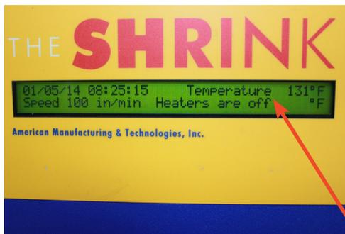
10. TO SHUT DOWN HEATERS: PRESS TEMP BUTTON AND ENTER "0" THEN PRESS ENTER BUTTON.
