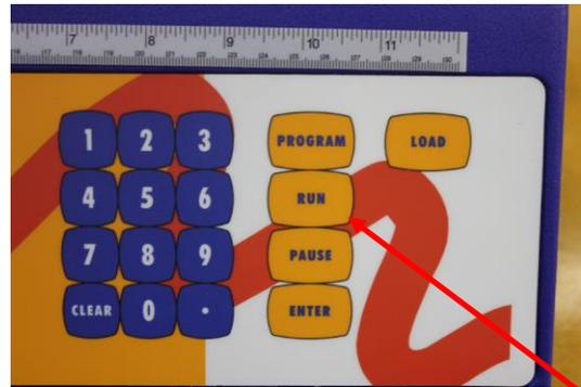
10. TO RUN, PRESS THE "RUN" KEY. MATERIAL WILL THEN BEGIN DESIRED MEASURING AND CUTTING PROCESS.
