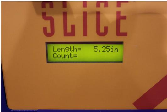
9. LCD WILL SHOW "Count=". ENTER RUN QUANTITY AND PRESS "ENTER" ON THE KEYPAD.
